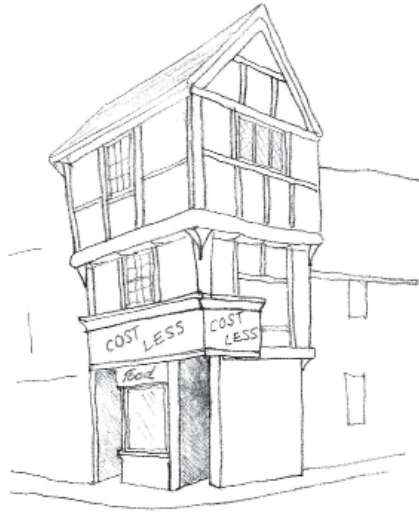
This shop front and fascia takes no account of scale or architectural style of host building
